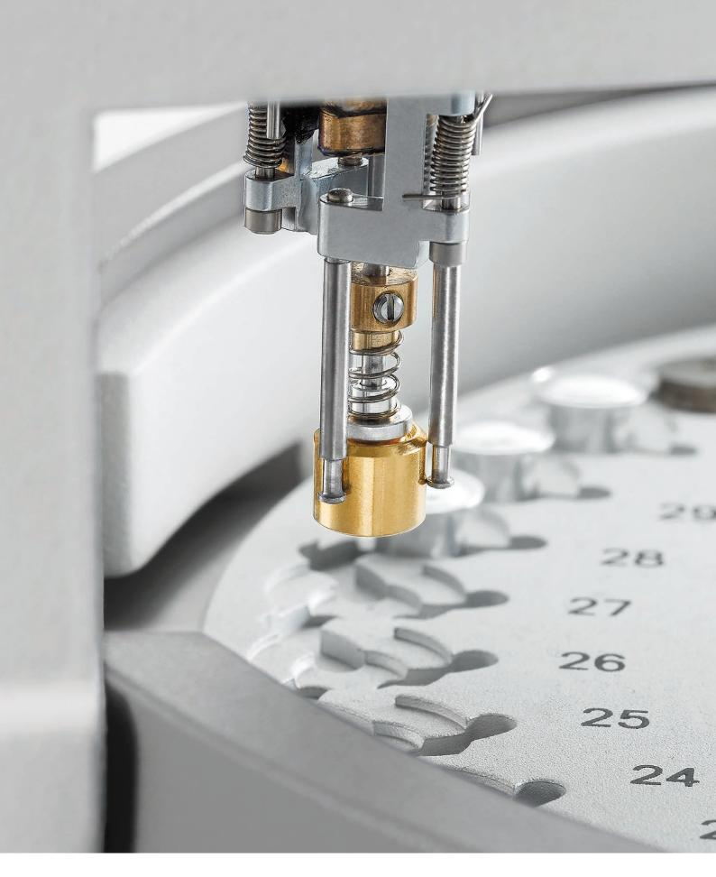
All our DSC and TGA models can be automated. The sample robot can handle any crucible in any sequence.
