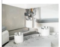
Even 900 µL crucibles can be handled by the robot (special grippers with a longer swiveling arm – ArtNo: 30293250 – are necessary). These special grippers are limited to TGA/SDTA (LF/HT) sensors.
