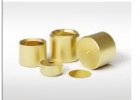
These HP gold-plated steel crucibles (25  $\mu$ L and 40  $\mu$ L volume) have proven highly effective in the field of safety investigations. These are the optimal single-use crucibles for a pressure up to 15 MPa. The crucible lid is pressed (pressure of about a ton) into the crucible with the aid of a special toggle press so that the rupture disk (gold) hermetically seals the crucible.
