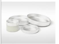
All alumina crucibles are provided with alumina lids. These lids have a hole. For applications with samples that contain volatile substances, drying out or moisture uptake is critical. For such cases, aluminum lids are available that can be removed by the sample robot before the crucible is transferred to the furnace.
