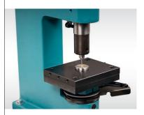
High-pressure crucibles ( $25 \mu L$  and  $40 \mu L$ ) can be sealed by using a special sealing press (Maeder press). A particular plunger/die set is included for these two types of crucibles.
