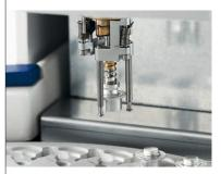
The lid piercing device (wasp) is a unique feature. Samples releasing volatiles or being hygroscopic can be enclosed in hermetically sealed crucibles to prevent mass changes prior to analysis. With the lid piercing kit hermetically sealed aluminum crucibles can be opened just before analysis in the DSC or TGA instrument.
