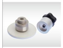
**B:** This assembly consists of a lower part to keep the hexagonal crucible and an upper part (turning head) that fits on the crucible cover. The crucible is closed with the seal disk by turning until a sliding clutch is activated. After the measurement, the crucible is opened with the same tool. ArtNo: 51119915
