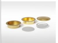
Gold or gold-plated crucibles (40 µL) are chemically resistant and the optimal choice if strong acids or bases have to be analyzed. These pans are the only non-aluminum types that can be hermetically sealed by coldwelding; maximum pressure: 0.25 MPa (gold) and 0.2 MPa (gold-plated Al).
