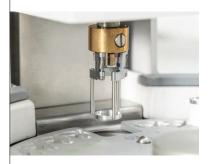
The sample robot can remove the protective aluminum lid from the alumina crucibles. It prevents loss or uptake of water of samples in alumina crucibles. It also protects oxygen-sensitive samples from oxidation.
